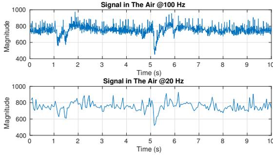
**Figure 3:** Comparison of different sampling frequency.
