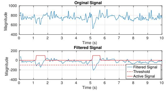
**Figure 4:** Filtered signal with active line.
