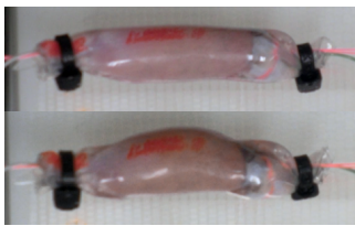
Figure 3: A biological muscle actuator which packaged physiological solution developed. Upper figure shows the natural state of the actuator. And the lower figure shows tetanic contraction by electrical stimulation.
