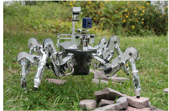
Fig. 1 LAURON IVc: Fourth generation of the bio-inspired (stick insect) walking robot LAURON.
