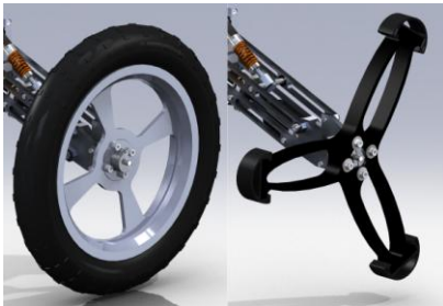
Fig. 3 Left: Different classic effectors are available for ROLV robot with a diameter of about 0.32 m. Left: Wheel effector. Right: Stiff hybrid wheel effector with three spoke-like elements
