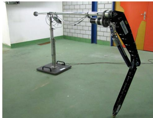
Fig. 1 Two segment hopping leg robot attached to a test rig with a passive spring in place of the actuator.
