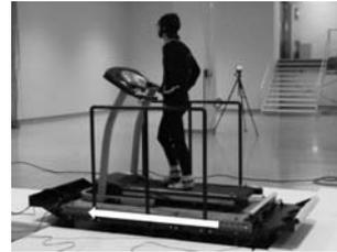
Fig. 1 Experimental device. Treadmill horizontally moves with servo motor equipped on the floor of the treadmill. Subjects walk on the treadmill suffering pulsed perturbation in arrowed direction once for one trial.
