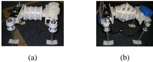
Fig.2 Robots equipped with rectangle (a) and rhombus (b) shaped tendon-driven actuated spine.
