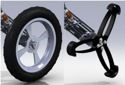
Fig. 3 Left: Different classic effectors are available for ROLV robot with a diameter of about 0.32 m. Left: Wheel effector. Right: Stiff hybrid wheel effector with three spoke-like elements
