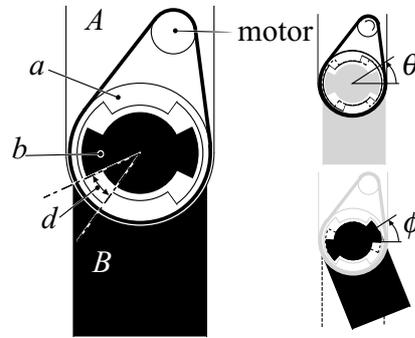
Figure 8: Principle of the backlash clutch
