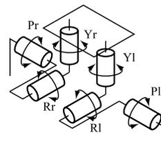
Figure 1: DOF arrangement of conventional hip joint
