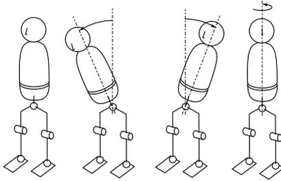
Figure 4: Bending motion of upper body with double spherical hip joints
