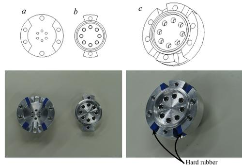
Figure 9: Components of the backlash clutch
