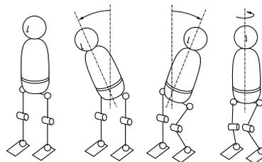
Figure 2: Bending motion of upper body with hip, knee and ankle joints
