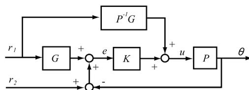
Figure 11: Two DOF control system
