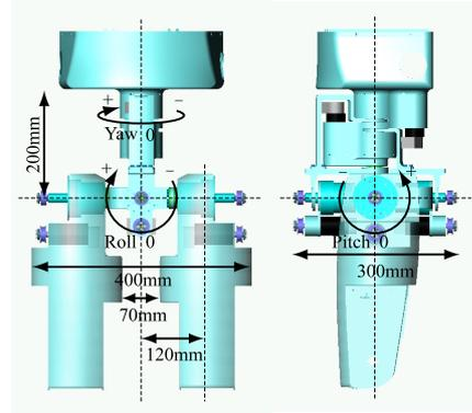
Figure 5: Dimensions of the designed double spherical hip joint
