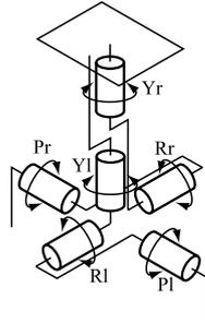
Figure 3: DOF arrangement of double spherical hip joint
