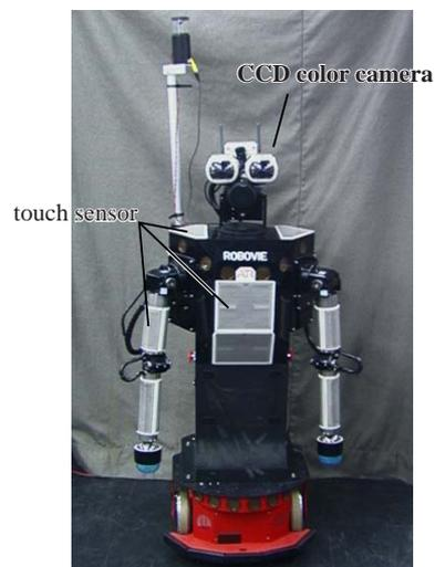
Figure 6: Humanoid robot Robovie
