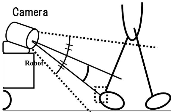
Fig. 5 Robot detected human's heel.
