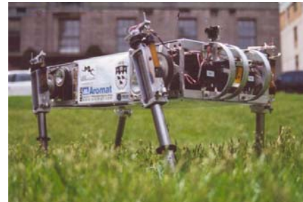
Figure 1. Scout II: A simple four-legged robot.
