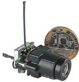
Fig. 4. The micro camera to be used for the PA10 robot
