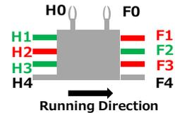
Figure 2: Reciprocal use of the legs in tripod running
