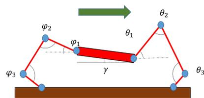
Figure 4: Transverse plane model: a serial 7-link model consists of the foreleg, the torso and the hind leg.
