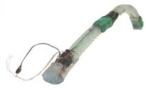
Some of these concepts have been implemented in a family of simple elastomeric robots (*Softworms*) and we have succeeded in generating caterpillar-like gaits based on model-free approaches using motion primitives and through distributed mechanical feedback. The next challenge is to make these robots climb in complex branched structures and to apply the control approaches to more diverse body shapes.
