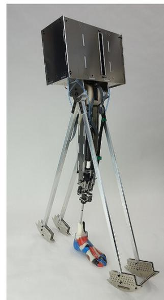
**Figure 4:** Pneumatically driven bipedal robot to drive cadaver foot.
