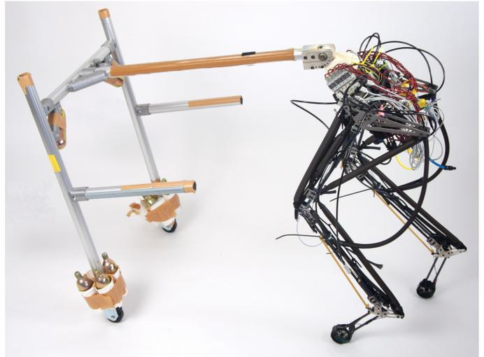
**Figure 1:** Picture of experimental setting with Pneupard's hindlimbs attached to a sliding strut.
