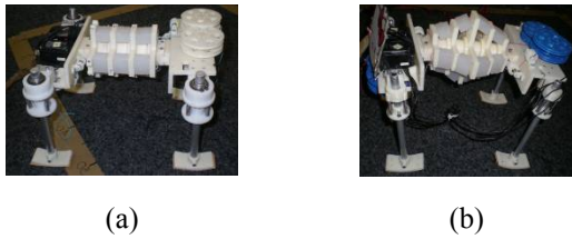
Fig.2 Robots equipped with rectangle (a) and rhombus (b) shaped tendon-driven actuated spine.
