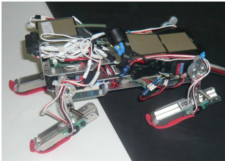
Fig. 1 **Quadruped robot used in case studies 1, 2.** A total of 12 sensors from 4 modalities (4 pressure sensors on feet, 4 angular sensors in passive knee joints, 3 acceleration sensors, and 1 infrared sensor) were used.
