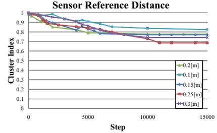
Fig. 6 The influence of the sensor reference distance
