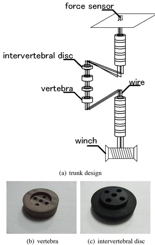
Fig. 2 Trunk design including redundant joints and tunable viscoelasticity
