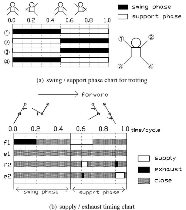
Fig. 4 leg operation for trotting
