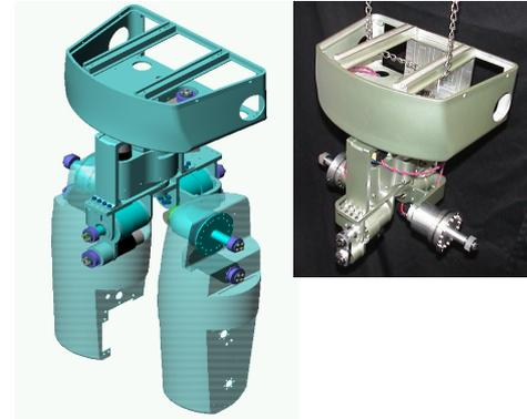
Figure 6: Photo of the double spherical hip joint
