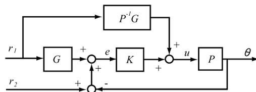
Figure 11: Two DOF control system
