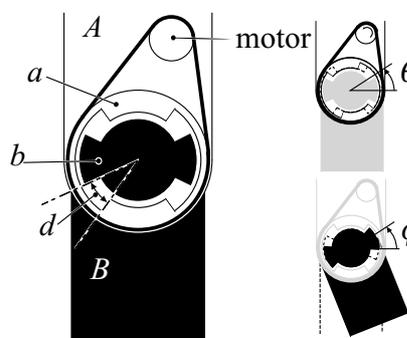
Figure 8: Principle of the backlash clutch
