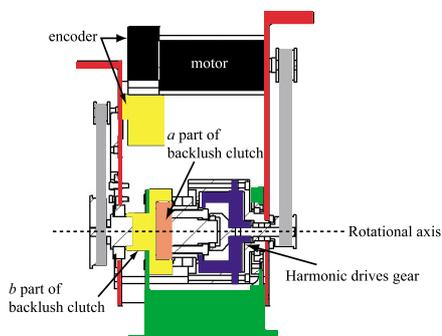
Figure 10: Design of the knee joint
