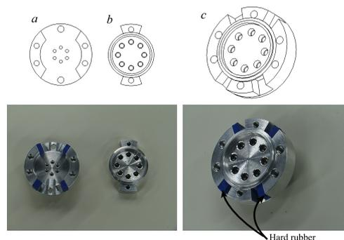
Figure 9: Components of the backlash clutch
