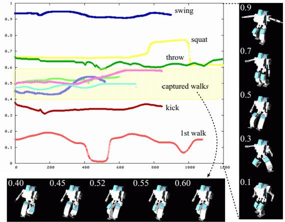
Figure 6: Internal representation of each motion pattern and corresponding attitude of humanoid robot.
