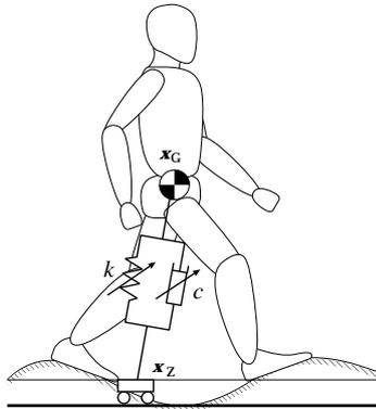
Figure 6: Legged system and VIIP model
