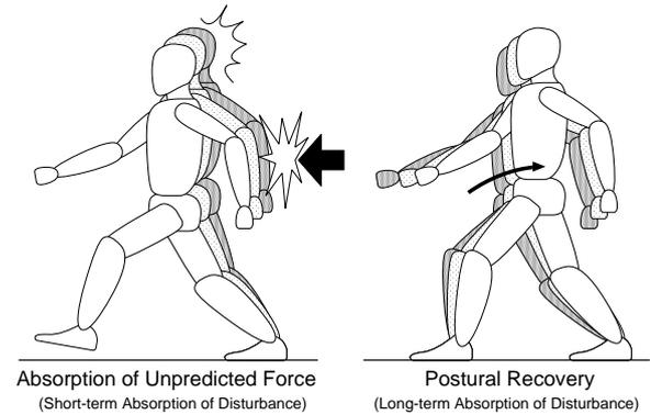
Figure 2: The two basic schemes to balance
