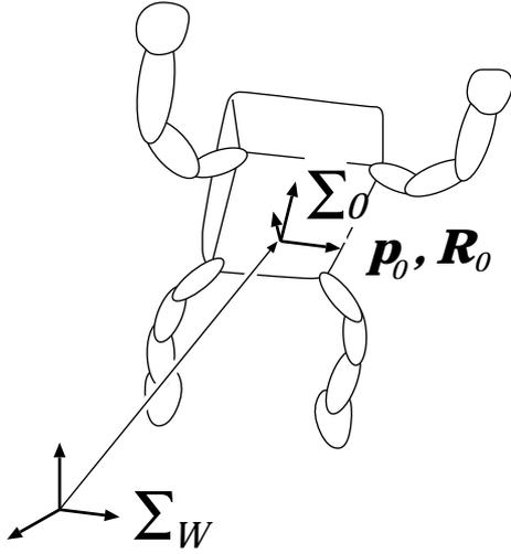
Figure 1: Multi-body Legged Robot
