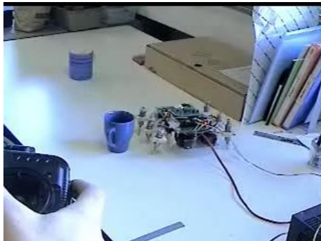
Fig.14 Robot locomotion by the radio control system
