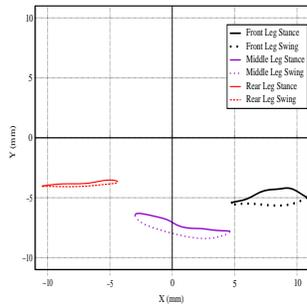
Figure 7: Foot trajectories for the three feet on the right side of the body, top view or  $X$ - $Y$  plane
