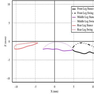
Figure 8: Footfall trajectory for three feet, side view or  $X$ - $Z$  plane
