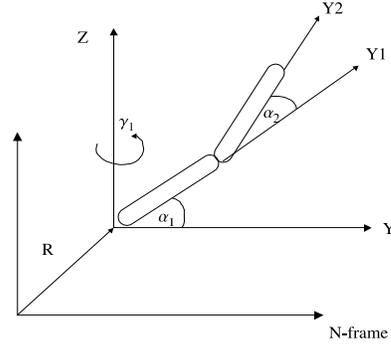
Figure 6: Two bar linkage represents the femur and tibia segments
