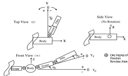
Figure 9: Leg angles measurement
