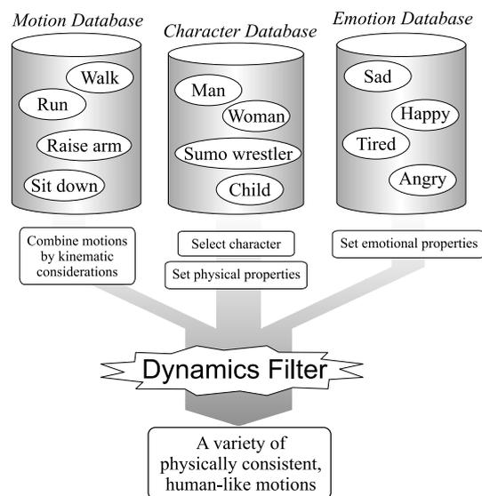
Figure 2: Motion generation via dynamics filter
