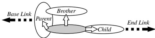
Figure 4: Three pointers to describe link connectivity
