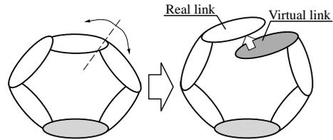
Figure 5: Virtual link to describe closed kinematic chains
