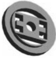
Figure 4: 2-DoF force/torque sensor wheel for elbow joint.
