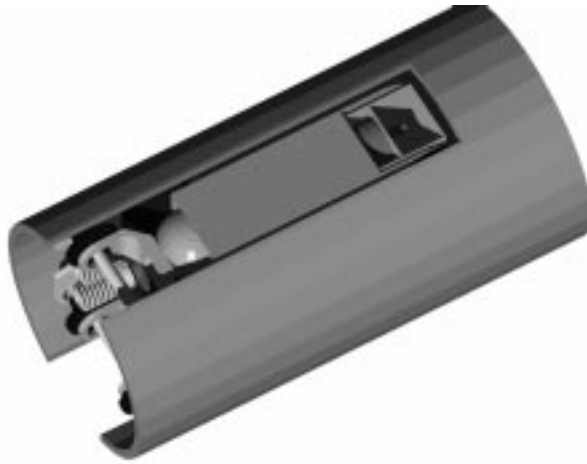
Figure 2: CAD rendering of TerminatorBot in the stowed configuration.
