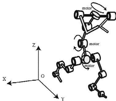
Figure 1: 3D biped robot
